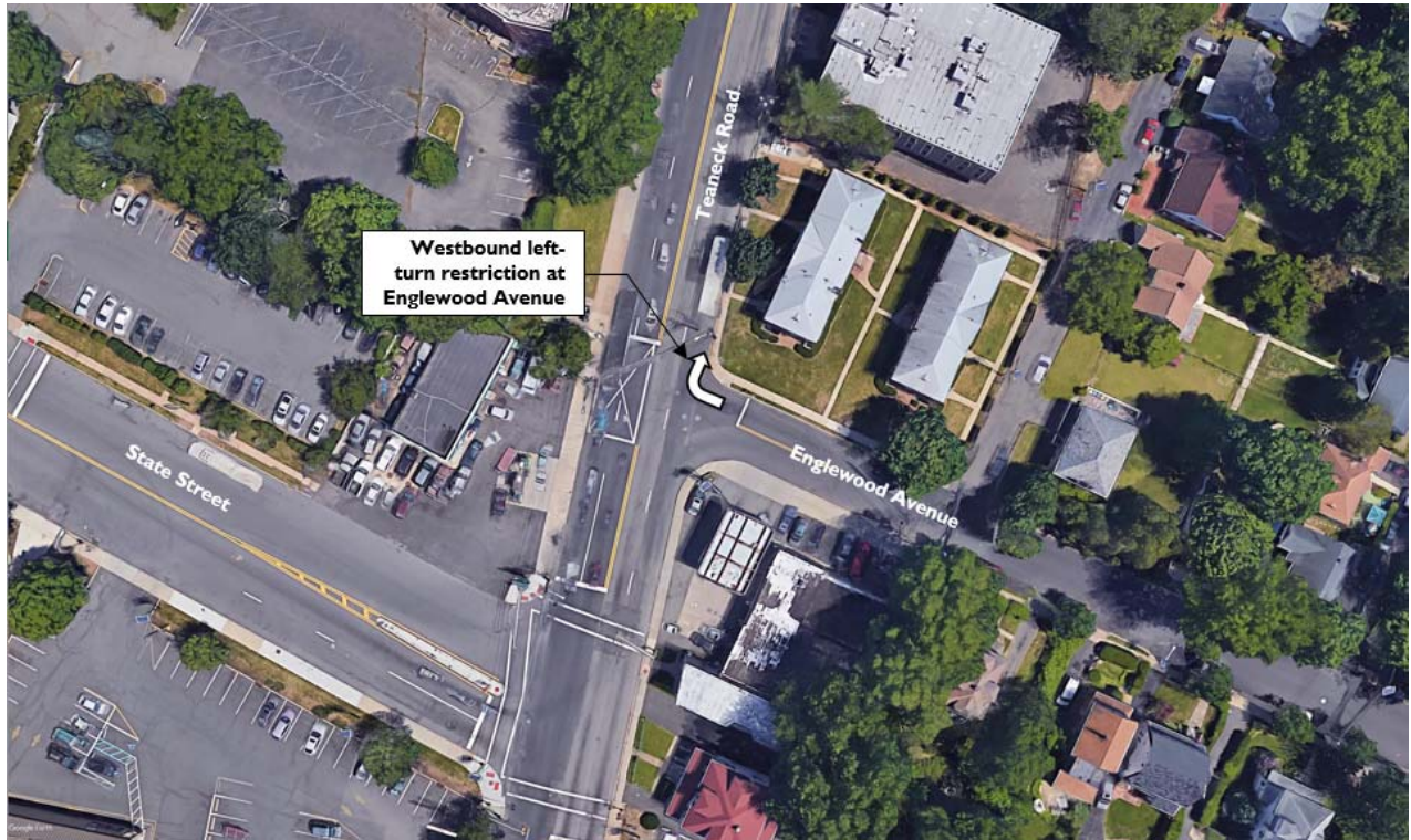
Figure 8: Westbound left-turn restriction at the intersection of Teaneck Road and Englewood Avenue
